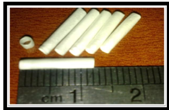
Fig. 1. Display of about 12-mm PLGA/ Nanosilver conduits intended to substitute a 10mm nerve gap.
