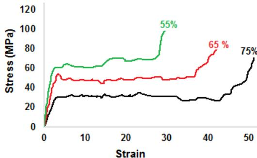
**Fig 3.** Engineering stress-strain curves of titanium scaffolds with 55, 65, and 75% porosity.
