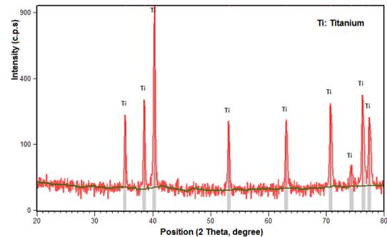
**Fig 2.** X-ray diffraction pattern for fabricated titanium scaffold.
